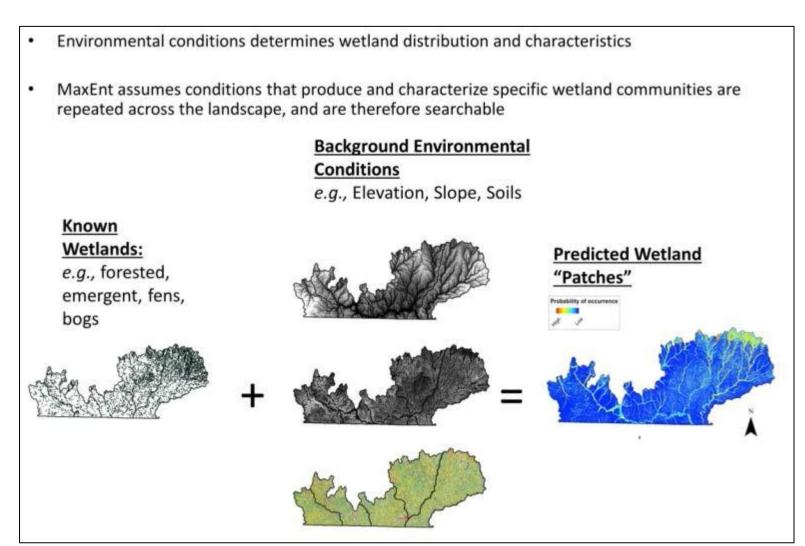
Figure 1: Description of how spatial modeling works when using Maxent, and other models types.
